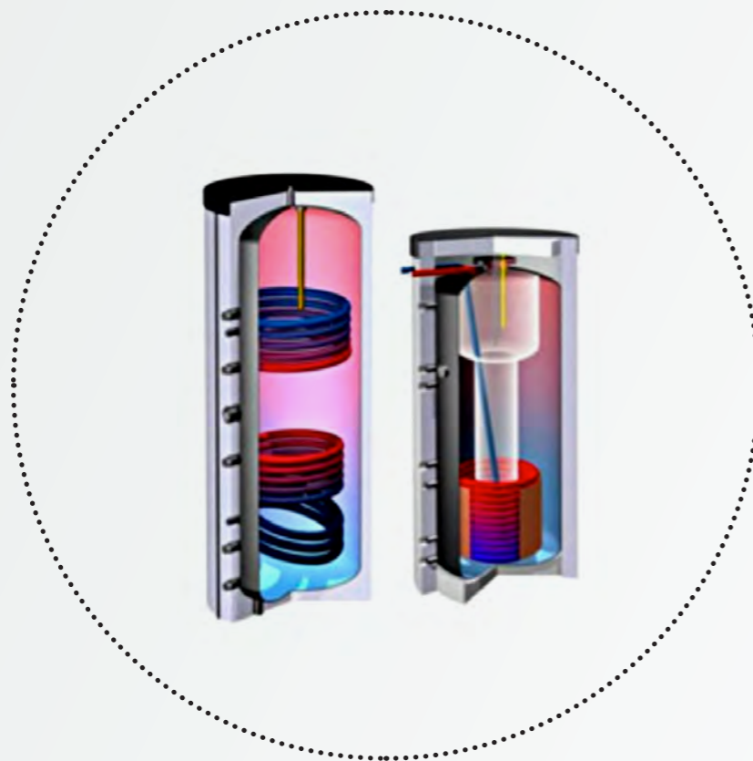
Single and double compartment water tanks for DHW and space heating
