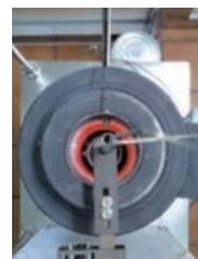
Non-flammability test (KS F ISO 1182)
