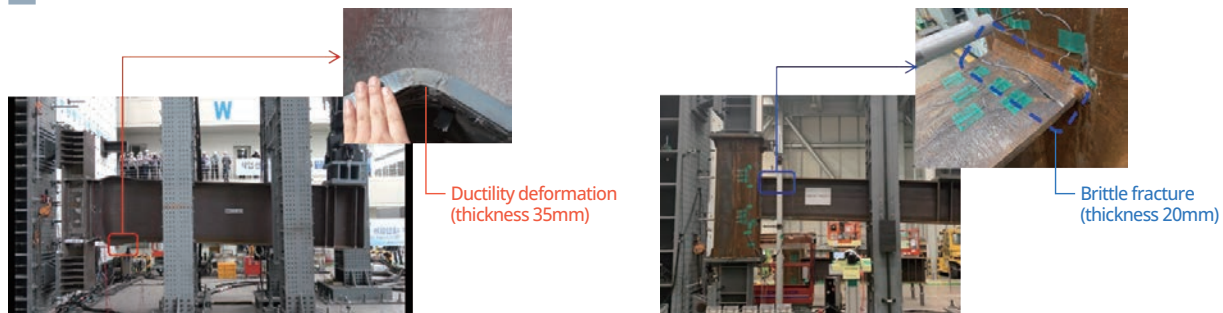
[Beam-column connection test using Pos-H] (PH-1,500mm 5% deformation → S.M.F)
