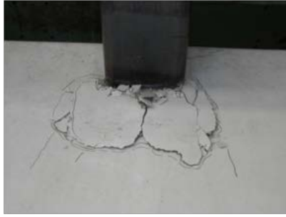
(a) Concrete crushing around the columns
