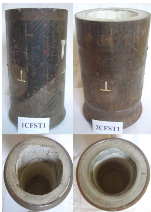
Fig 13. Single- and double-layered H-CFST tested specimens
