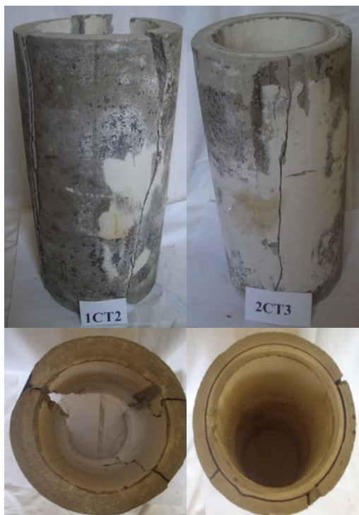
Fig 14. Single- and double-layered H-CT tested specimens
