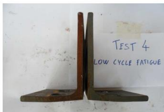
Figure 67. Connection typology 1: dissipative link specimen and angle profiles after the test
