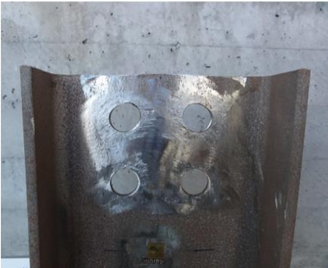
Figure 69. Connection typology 2: dissipative link specimen after the test
