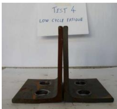
Figure 67. Connection typology 1: dissipative link specimen and angle profiles after the test
