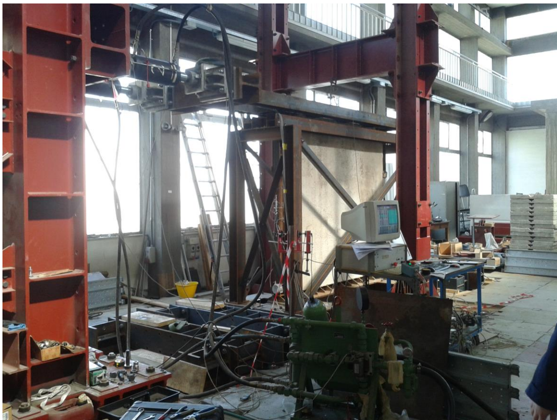
Figure 83. Testing of the downscaled SRCW specimen
